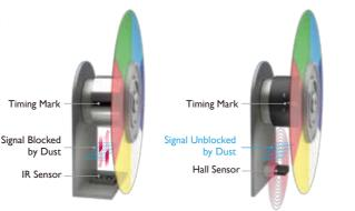
\* After experimenting in the same environment, hall sensor maintains normal functionality even after having 40g of sand inside, whereas traditional sensor loses its detection capacity after having 6g of sand inside.
