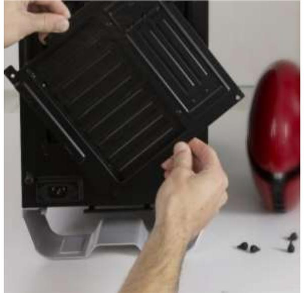
Rotatable PCI Bracket Window
