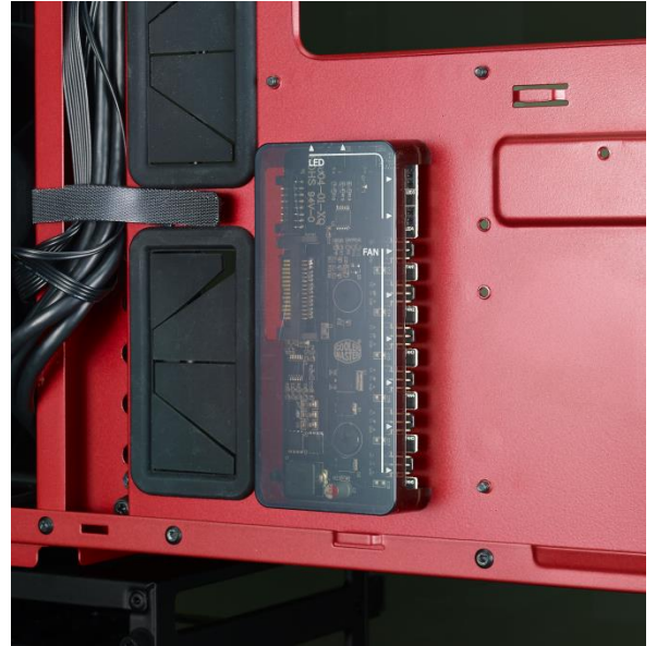
Fans and LED control board specific to our MasterCase Maker models
